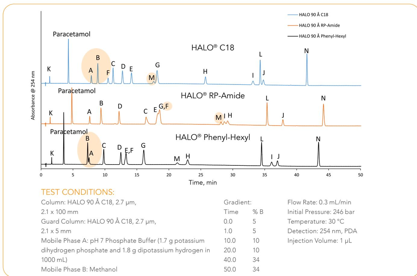
Figure 7. Paracetamol and associated impurities screened on HALO® C18, HALO® RP-Amide, and HALO® Phenyl-Hexyl.
