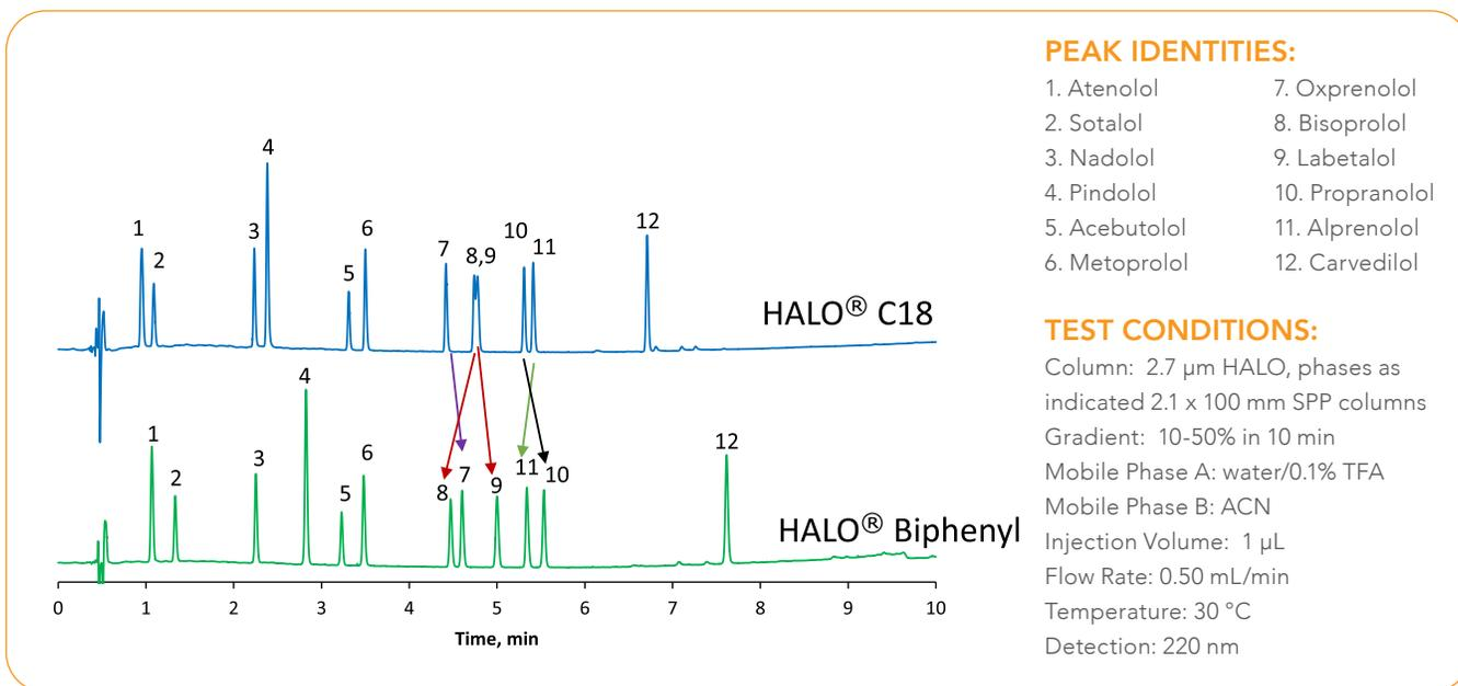
Figure 3. Comparison of  $\beta$ -blocker separations on HALO<sup>®</sup> C18 and HALO<sup>®</sup> Biphenyl.
