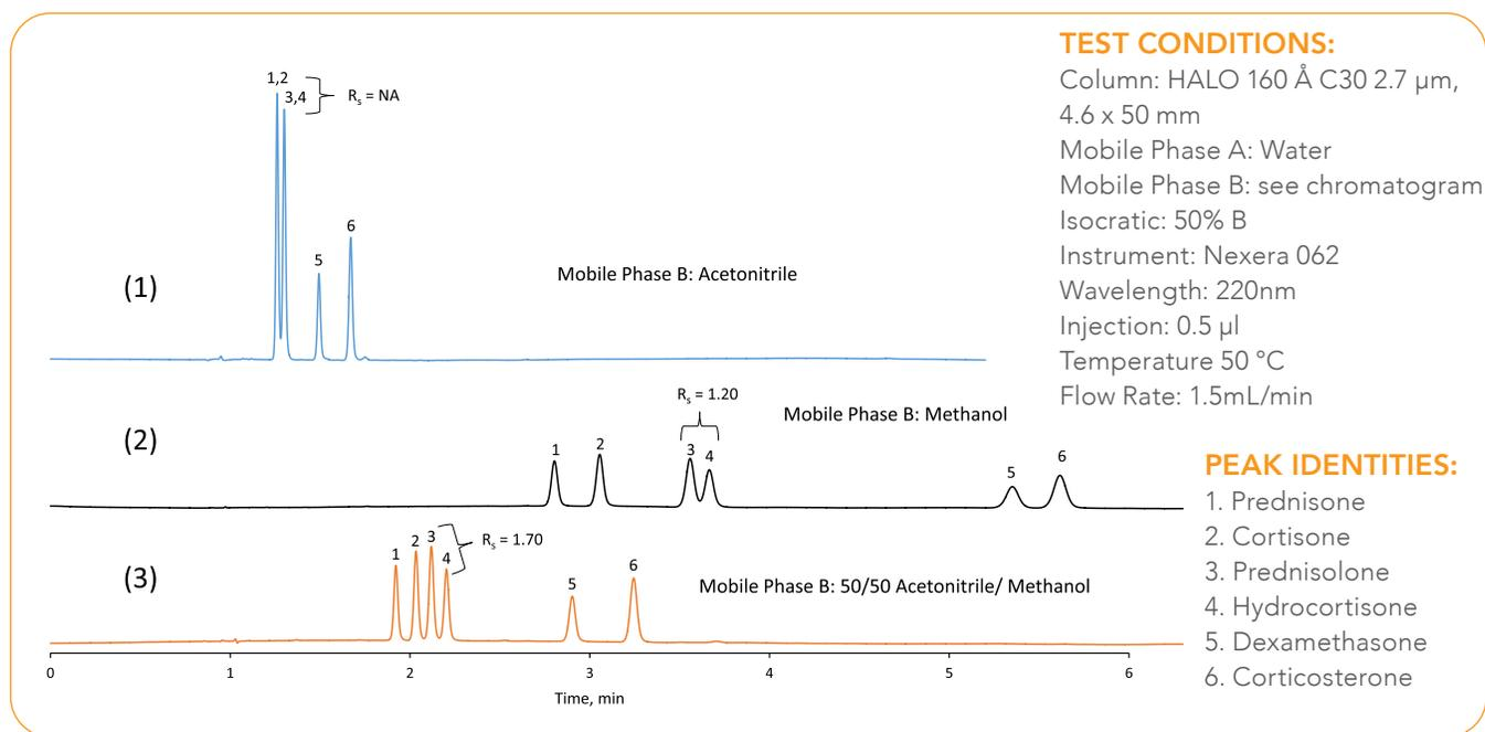
Figure 4. Effect of different mobile phase solvents on the separation of steroids.
