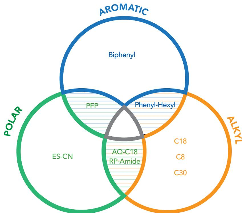
Figure 5. Chemical classification of HALO® reversed-phase stationary phases.
