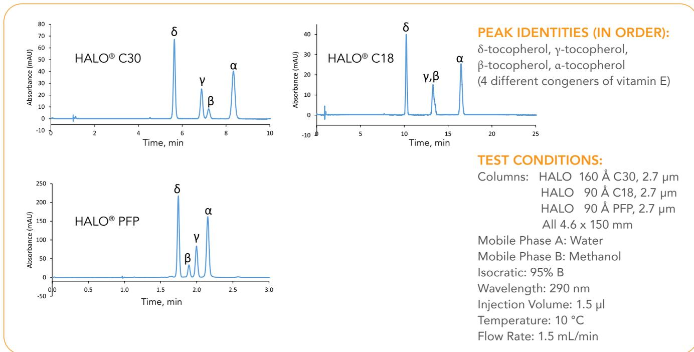
Figure 8. Tocopherol separation screened on HALO® C30, HALO® C18, and HALO® PFP.
