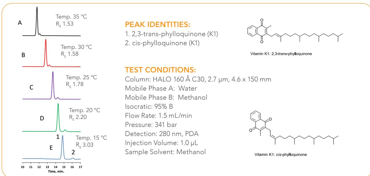
Figure 10. Effect of temperature on resolution using HALO® C30.
