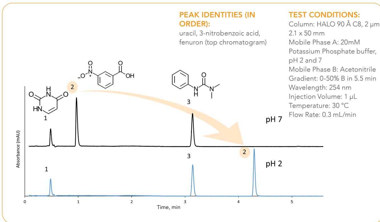
Figure 9. Effect of pH on retention time.
