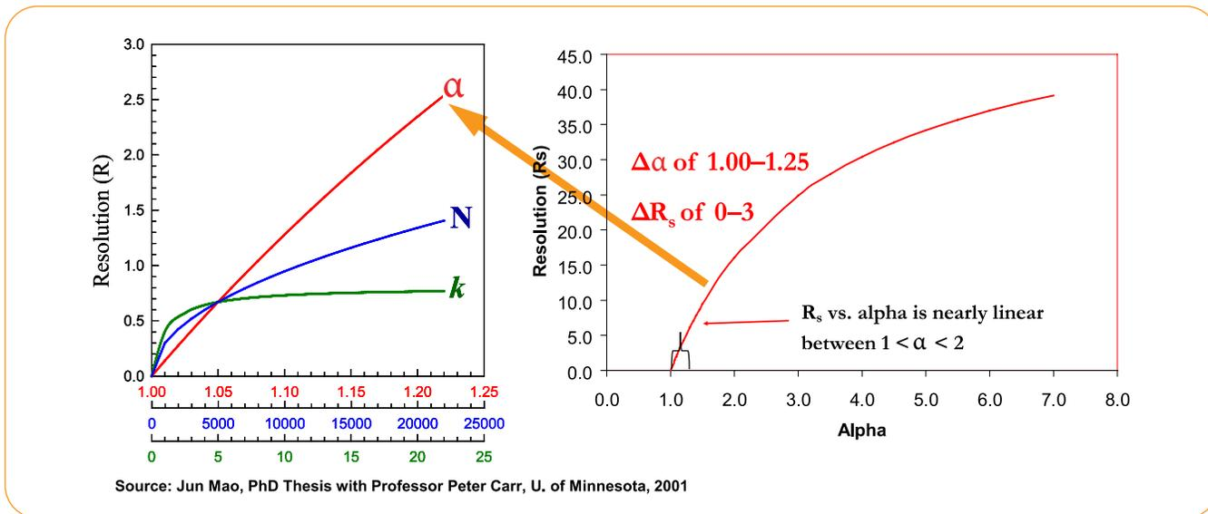
Figure 2. Plot of resolution vs. selectivity (red), efficiency (blue), and retention factor (green).
